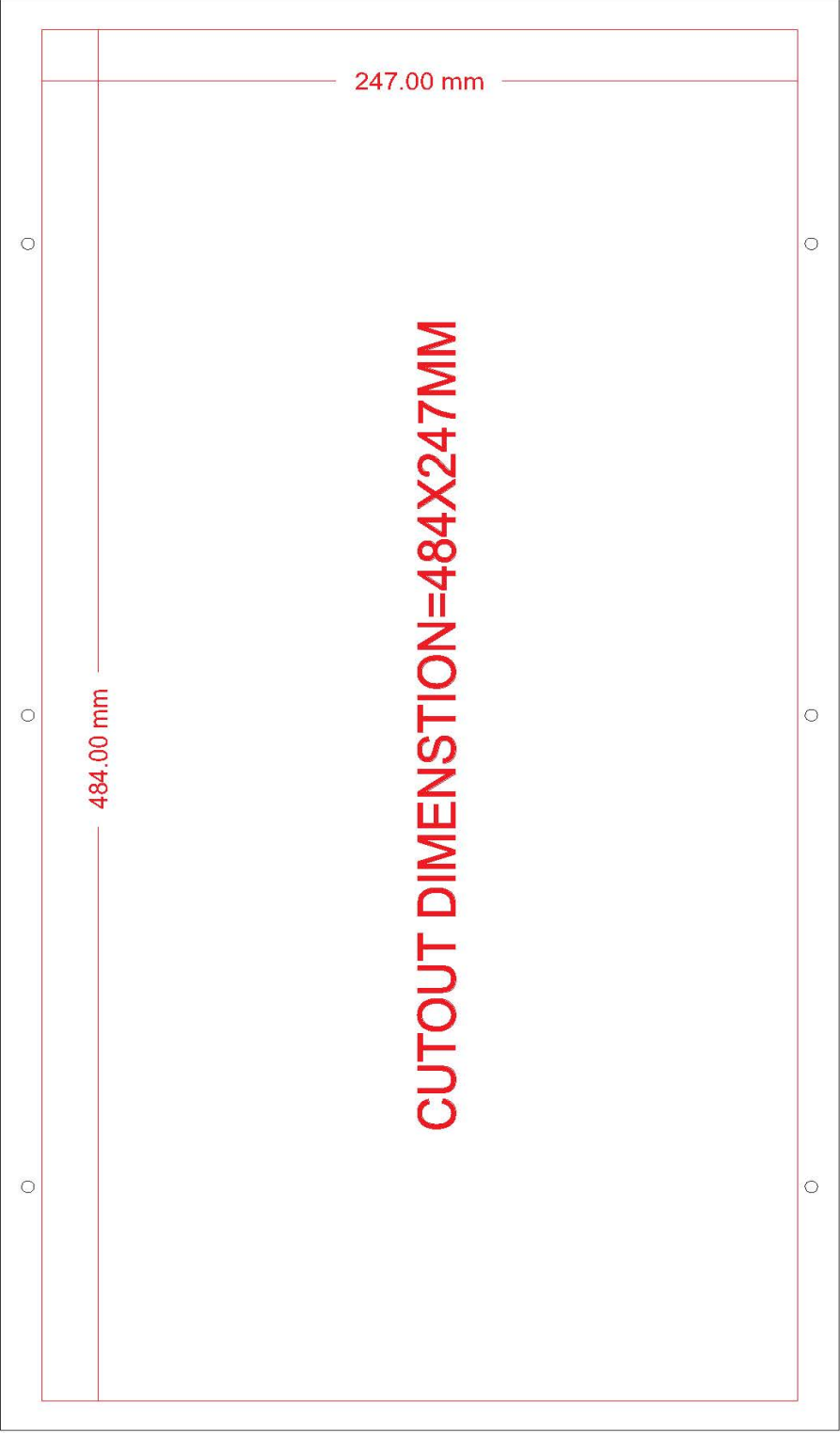
Cutout Dimension:- Height 484 mm X width 247 X Depth 63mm
